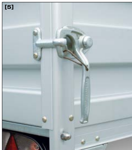
Safe loading: The large, solid lever locks allow quick loading and unloading of the trailer.
