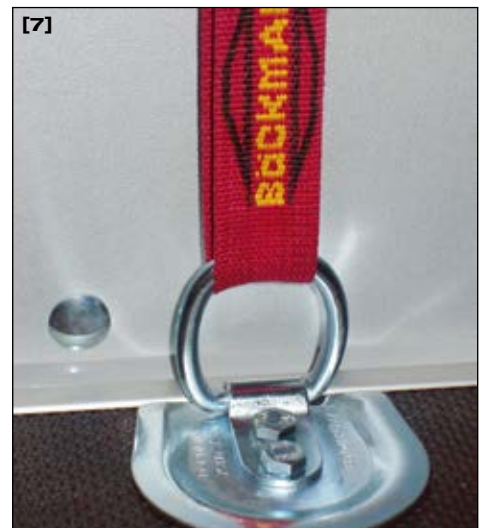
Safe travelling: The lashing rings bolted securely to the screen printed flooring enable you to safe load securing
